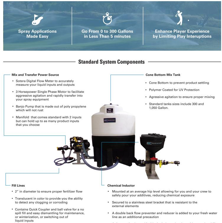
• A rinse station located inside the inductor bowl provides you the ability to thoroughly rinse your containers with fresh water and add back into your tank mixture without having to separately triple rinse
